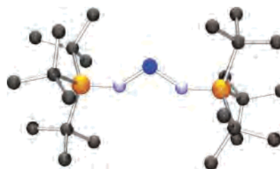
Figure 3. POV-ray drawing of 6 . Color code: C, black; N, light blue; B, blue; P, orange. H atoms are omitted for clarity. Selected distances (Å) and angles (deg): P–N 1.535(7), B–N 1.41(5), N–B–N 117(2), B–N–P 148.2(16).
